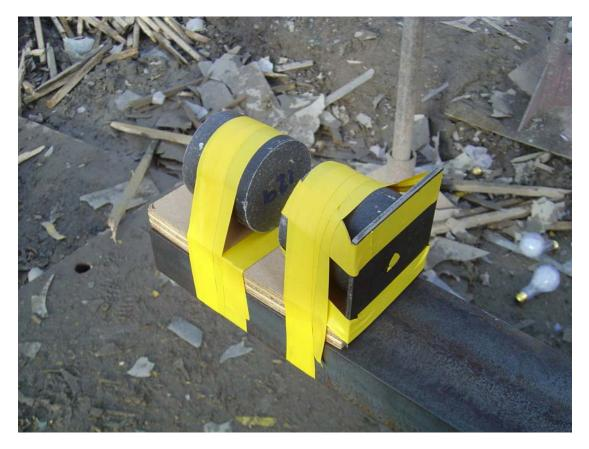
Figure 3. Experimental Set-Up for an XDT experiment with 2 ROWANEX 3000 charges and a steel cover plate.
