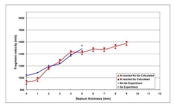
Figure 2. Plot of the response for ROWANEX 1400 with aluminium cover plates attacked by 13.15mm projectiles. The experimental data is shown in blue and the predicted values, using CHARM, are given in red.
