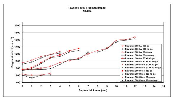
Figure 1. Experimental data for ROWANEX 3000 firings employing 13.15mm, 20mm and STANAG 4496 (14.3mm diameter) projectiles through both aluminium and steel barriers.
